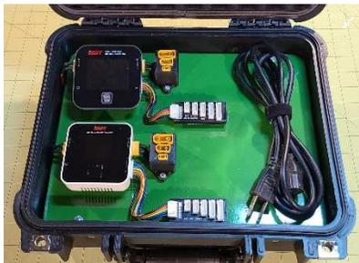
All the fittings and wiring were assembled for the final time. The chargers and balance boards are attached to the plywood plate with some Scotch brand Extreme Hook & Loop Fasteners.
