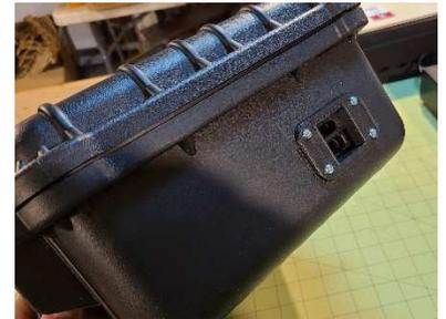
I knew that trying to solder connectors once installed in a 3D printed part would be tough to do without distorting the printed piece. I made as many solder joints as possible prior to installing the connectors in the brackets. I still had to make a couple of connections on the charge block after the connectors were in place. It can be done without overheating the printed part, you just have to be careful.
